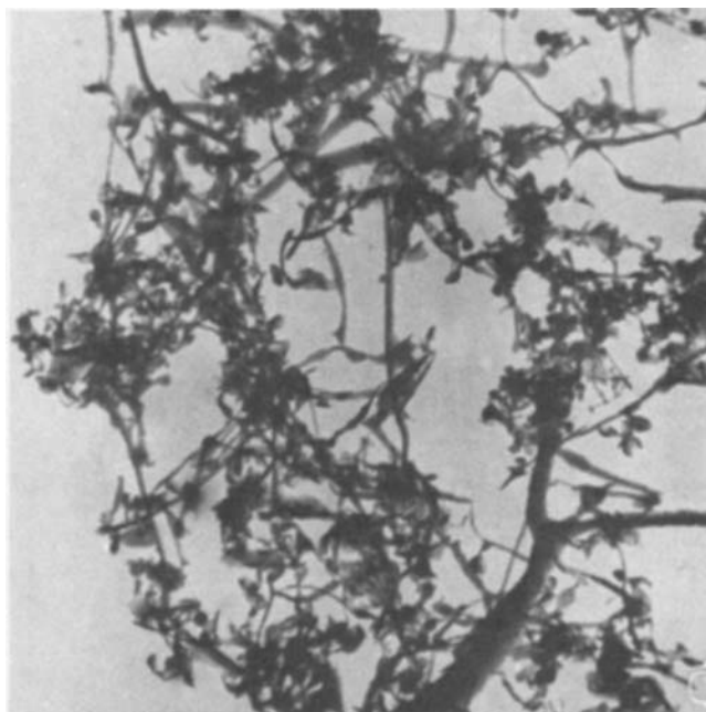
Fig. 3b. Stages in the formation of spherical particles—polymeric species formed during evaporation, 4000X.
